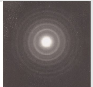
Fig. 9: Debye-Scherrer pattern of a powdered sample of CsCl. Thickness of the sample: 0.4 mm. Ex-posure time: 2.0 h.
