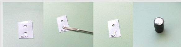
Fig. 7 a-d: sample preparation, a: perforated paper (3 layers) with adhesive tape; b: filling in the powder; c: smoothing the surface; d: fastening on the diaphragm tube
